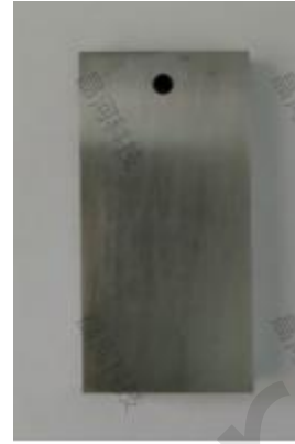
Fig.2.11-22 45# Initial state of the sample Fig. 2.11-23 100°C&50%RH/24h Fig. 2.11-24 45# State after cleaning CR TM-SGrease-1450N Metal corrosion test results
